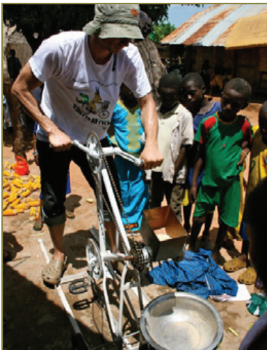
Engineer Tim Johnson demonstrates the use of his pedal-powered grain mill.
